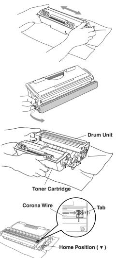
8 Reinstall the drum unit and close the front cover.
