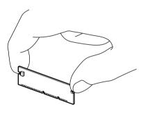
Make sure the memory board is securely seated on the main controller board.
