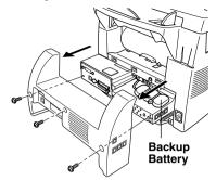
**3** Remove the screws securing the access plate and remove the plate.
