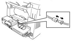
**5** To install the memory board onto the main controller board, plug the attached spacer into the connectors of the main controller board.
